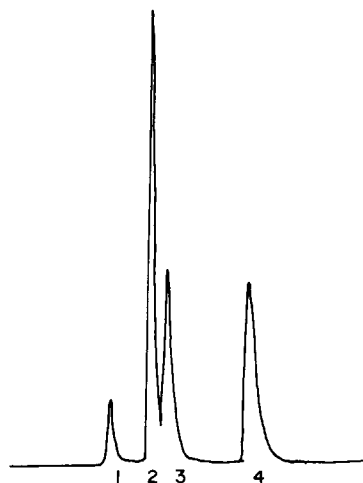
Fig. 2. Chromatogram for analysis of an NaBH 4 synthesis. 1 = CH 3 OH; 2 = (CH 3 ) 2 CO; 3 = (CH 3 ) 2 CHOH; 4 = CH 3 (CH 2 ) 2 OH.
